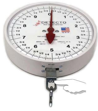
IF POINTER IS NOT AT ZERO, TURN THIS SCREW TO LEFT OR RIGHT.
