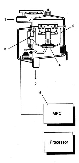
The milk enters the meter from above (1) and is collected in the metering cup (2). The cup is connected to a strain gauge (3) which senses the weight.
