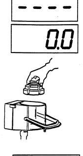
The MPC first displays "——", and then "0.0" for no weight; cup is empty.
