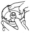
Remove the valve guide from the metering cup by pressing the wings outwards while pulling upwards (4).
